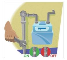
To isolate a ball valve, the handles needs to be turned in a clockwise direction so the arm is right angle to the rise piper.
